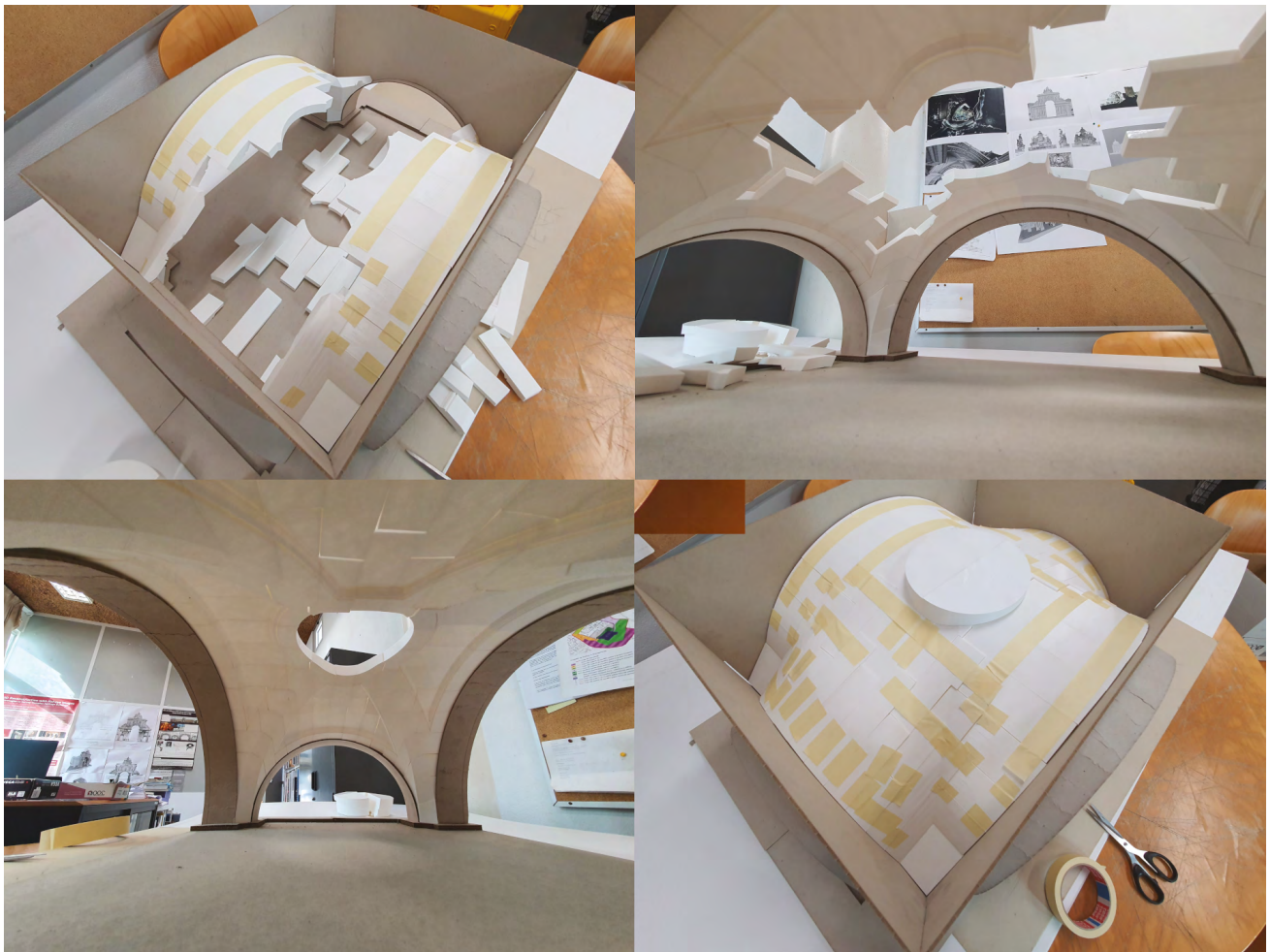
Fig. 25 Process of assembly of the voussoirs after 3D printing. Source: author, 2024.
