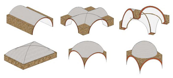
Fig. 6 3D library of parametric vaults modelled in Autodesk Revit 2024. Source: authors, 2024.
